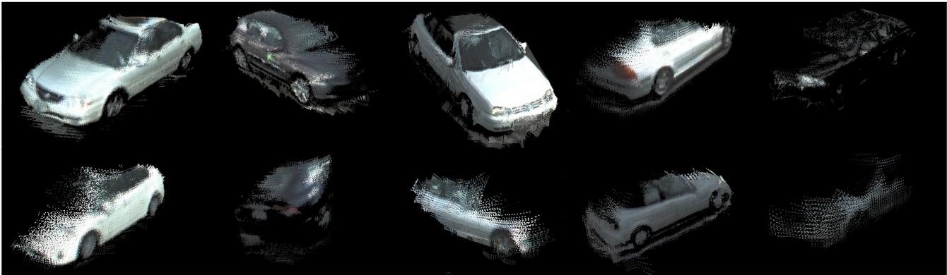
Fig. 5. Car models built using our interpolation and color-augmented grid search method, obtained from both moving and stationary cars.
