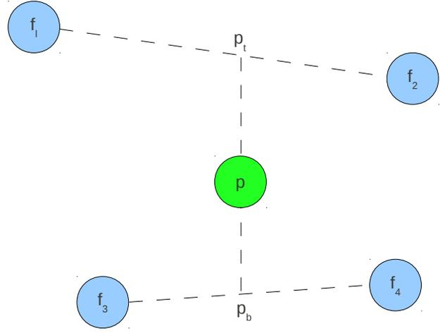
Fig. 3. Diagram of the bilinear interpolation used to estimate the 3D position of an image pixel  $p$ , shown in green. The 4 nearest surrounding laser points projected onto the image are shown in blue. First, the top 2 nearby laser points are linearly interpolated to get  $p_t$ . Next, the bottom 2 laser points are linearly interpolated to get  $p_b$ . Finally,  $p_t$  and  $p_b$  are themselves interpolated to get the final 3D position estimate for the pixel  $p$ .
