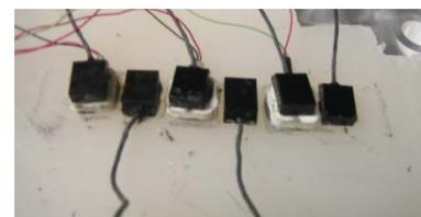
Figure 1. Tactors (white) mounted on the viscoelastic substrate (Skinsim) with accelerometers (black) mounted on the factors and Skinsim to measure movement when the factors are activated.
